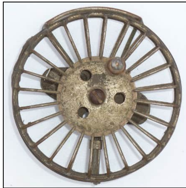
Top and bottom views of the museum's Vogel reel, likely a prototype designed by Seth Green and produced by John O. Vogel. Note use of the modified Billinghamurst Y-shaped support apparatus, visible on the bottom of the reel.
